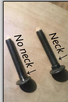
↓ Removing square neck with bench grinder ↓
