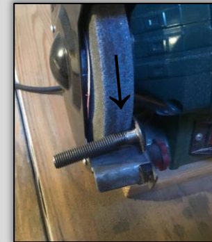
↓ Removing square neck with bench grinder ↓
